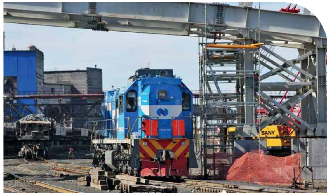
< The TEM18DM diesel locomotives perform shunting operations at the stations of the Technological Rail Transport Enterprise
